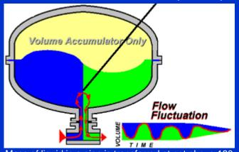
Mass of liquid in a pipe is transferred at not above 180 inches/sec or say 460 cm/sec
